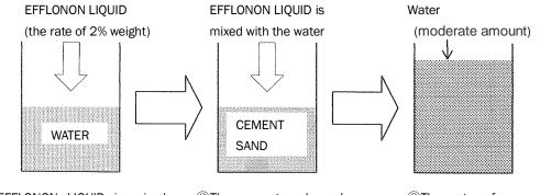
EFFLONON LIQUID is mixed with the water for mixture in cement together. ②The cement and sand were mixed. With ① is mixed
